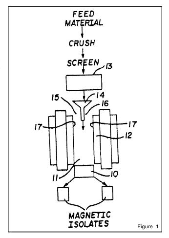
magnetic forces from first principles. With this method, the iron-based Frantz electromagnet can be used conveniently at up to full field strength to carry out analytical separations of feebly magnetic material. No assumptions are required and calibrations employing cumbersome standard materials are avoided.
